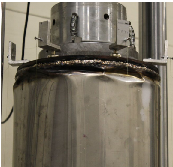
Figure 22. Bonded Specimen – End Crushing (Left) and Ring Stiffener (Right)
