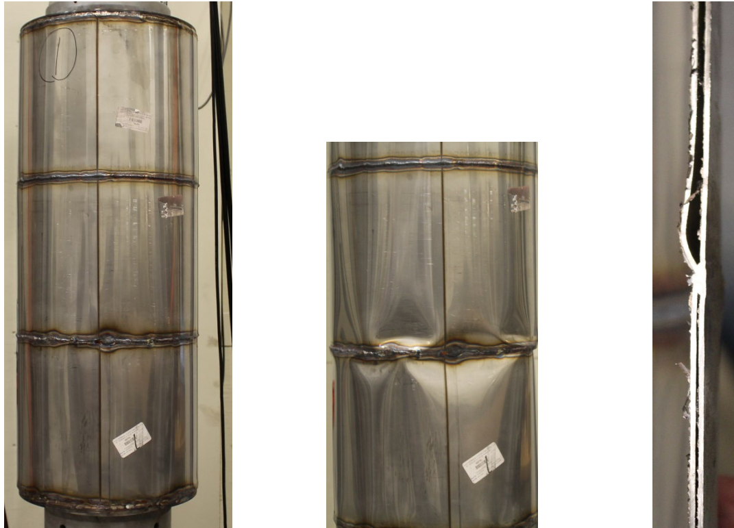
Figure 20. Visible Flaw (Left), Premature Buckle (Center), Cross-Section of Weld Flaw (Right)
