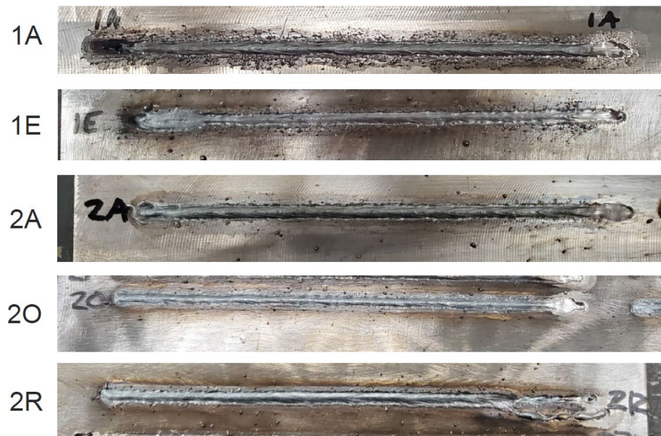
Figure 56. Bead On Plate Trials to Approximate HLAW Parameters
