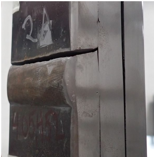
Figure 50. Specimen 2-A – Failure of 1st Layer (Left & Right Views)
