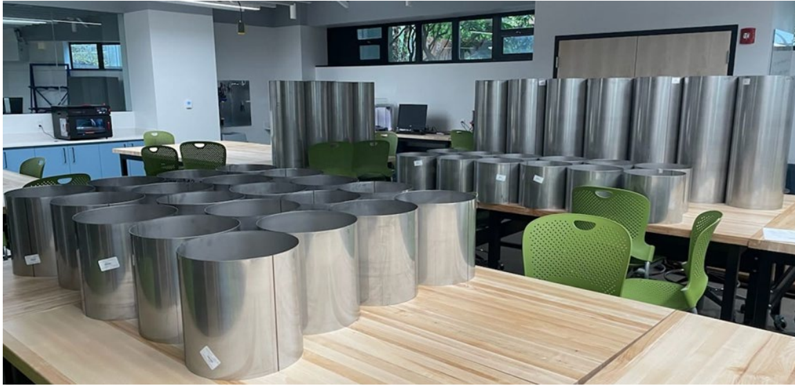
Figure 18. Benchtop Scale “Pipes” and “Sleeves” for Multi-Wrap Buckling Tests
