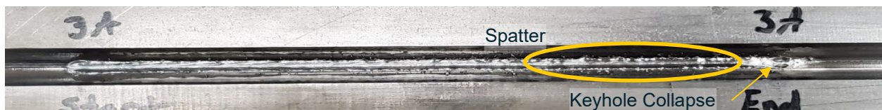
Figure 57. HLAW Trial #3A on U-Groove Joint – Above View (Top), Below View (Bottom)
