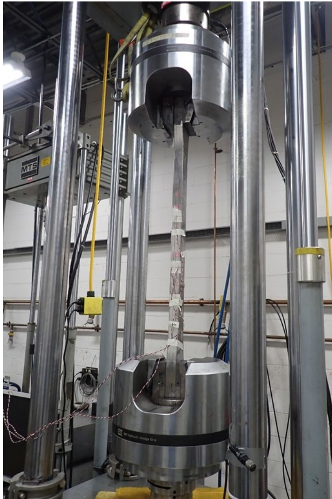
Figure 48. Fatigue Sample Instrumented and Loaded in the Test Frame
