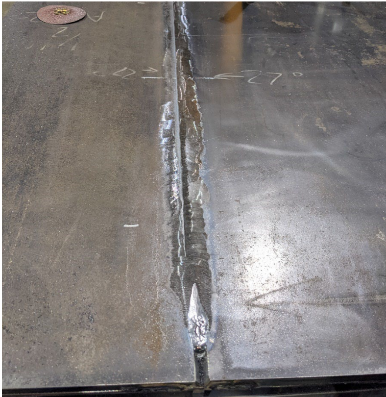
Figure 38. Remove Cap by Grinding
