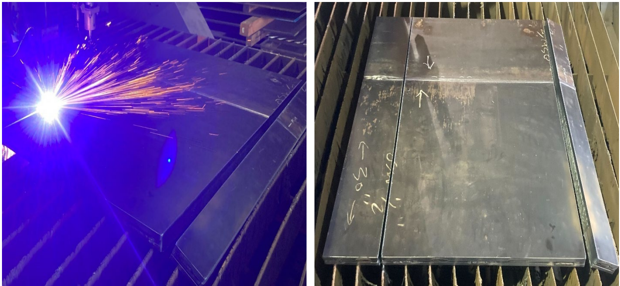
Figure 39. Plasma Cut Lead-in & Run-out of Completed Panels (Left) During Cut (Right) Complete
