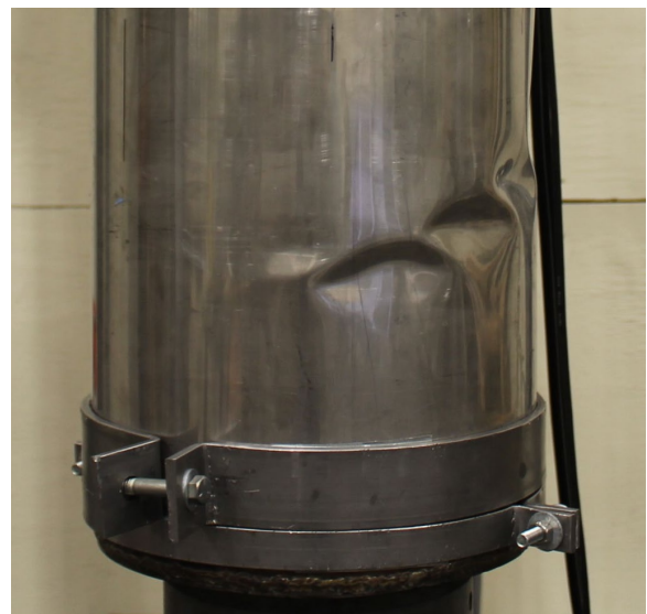
Figure 22. Bonded Specimen – End Crushing (Left) and Ring Stiffener (Right)
