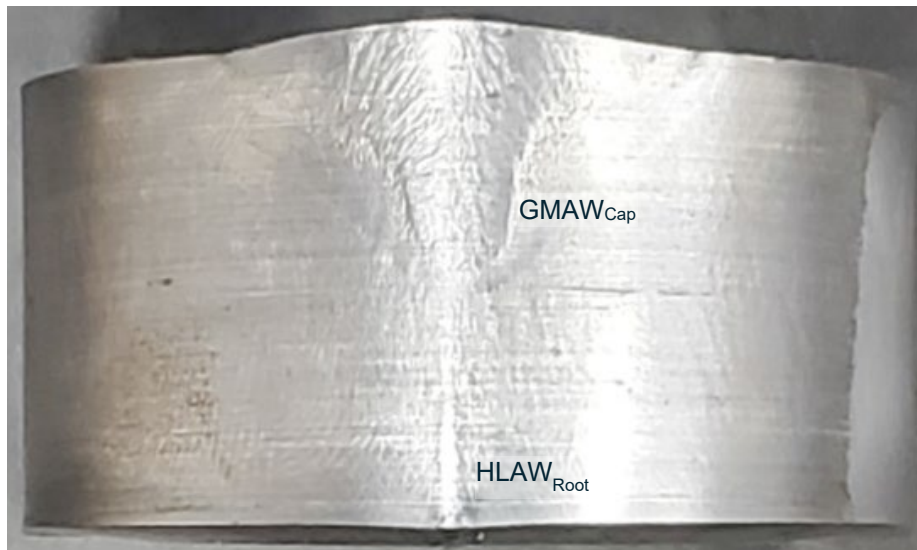
Figure 66. No Visible Defects on Bend Samples
