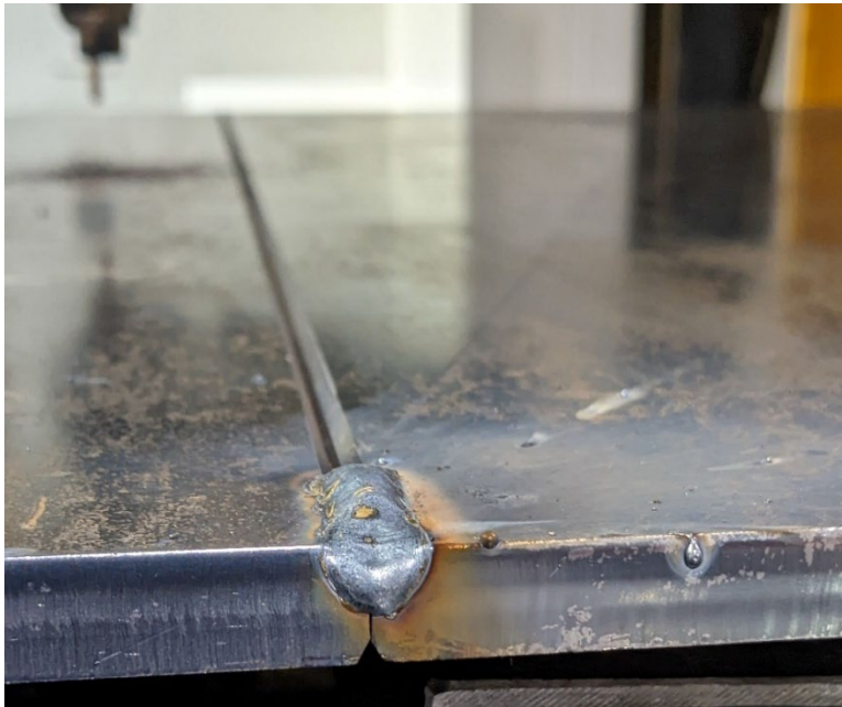
Figure 34. First Layer Butt Weld Joint Profile and Handling Tack Weld
