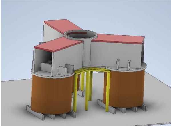
The Main Girder Top Plate will need to be built in precast sections. The issue with forming up the top plate in place is there would be no way to get the scaffolding out. Instead, each of these panels will be made in two parts and raised into place. These will all be held on with a closure pour.
