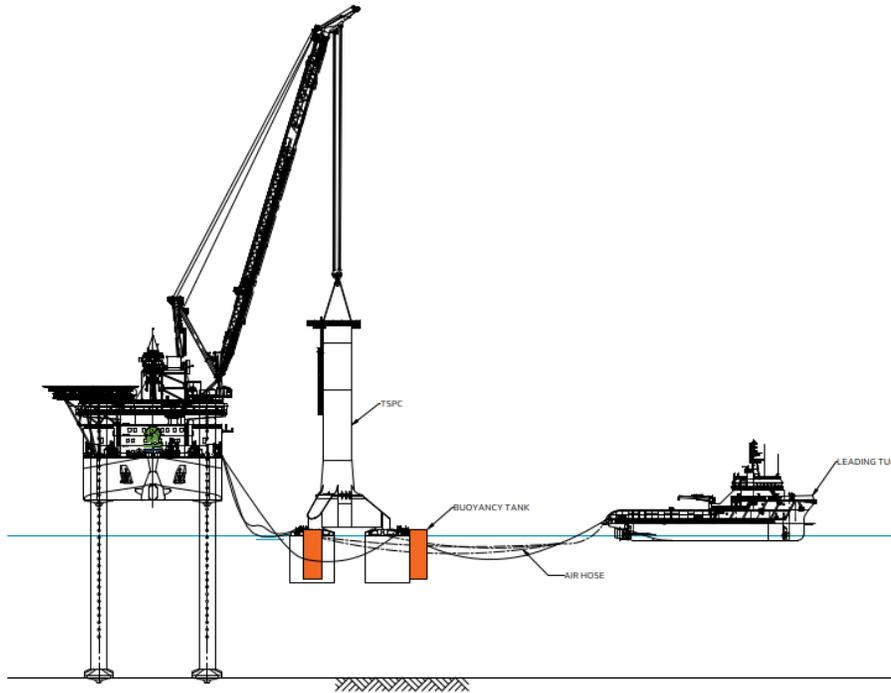
Step 4: Suction operation completed. Disconnect rigging, retrieve air hoses, suction pumps and buoyancy tanks.
