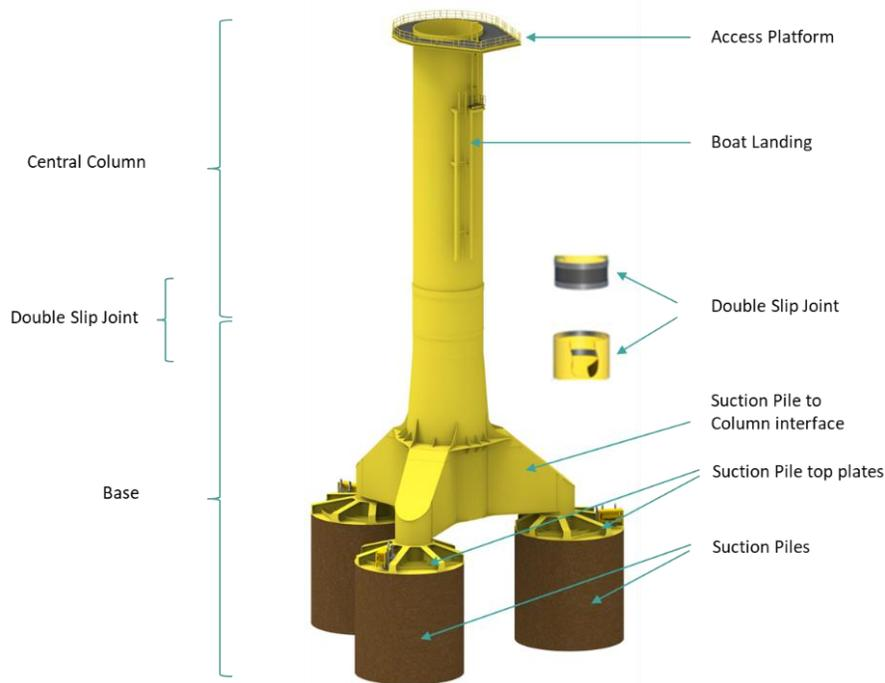
**Figure 3. TSPC – terminology of components – concrete version**
