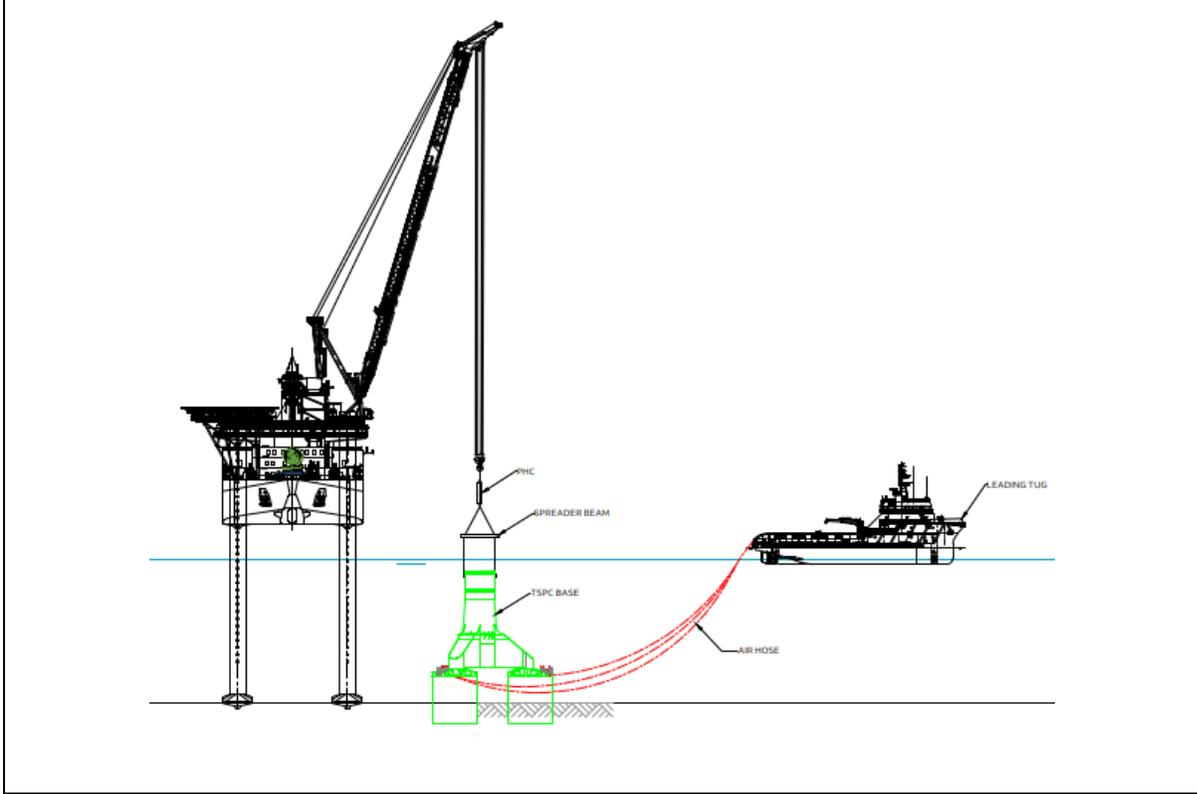
Step 5: Suction operation completed. Disconnect rigging, retrieve air hoses, suction pumps.
