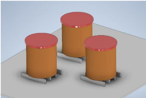
After the completion of cylinder lids a bracing system will be set into place. This bracing system will be made up of the same 24x84WF beams and have smaller stringers in-between. This will be set 15 m in the air with nine 0.9 m steel cylinder pipes. There will be additional support between the posts and some between the posts to the cylinder for rigidity purposes.
