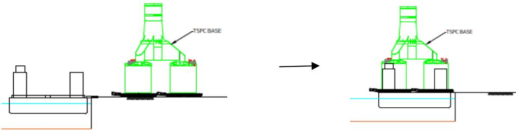
Step 2: Tow out the free-floating base with tugs directly to field OR tow out semi-sub barge to deeper waters, submerge the barge and tow out free-floating TSPC base.
