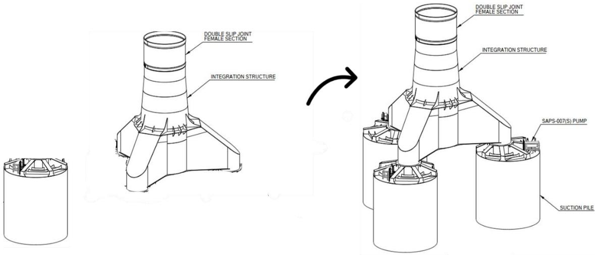
Figure 17. Final assembly of central column
