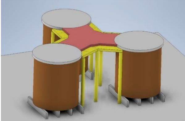
The middle concrete cylinder (highlighted in red) will be formed up with an inside form, the cage premade on the ground will be lifted into place, the outside form would be set, and the cylinder poured. After being poured the forms will be stripped and removed.
