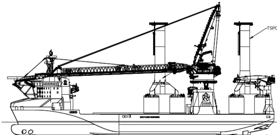
Step 3: Lower TSPC till self-weight penetration reached. Disconnect hoses. Start suction operation.
