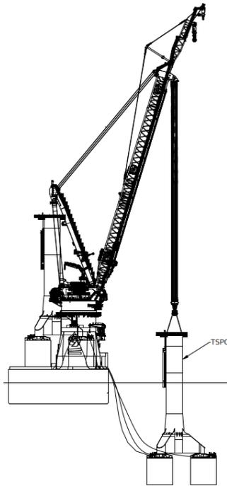
Step 4: Suction operation completed. Disconnect rigging, retrieve air hoses and suction pumps.
