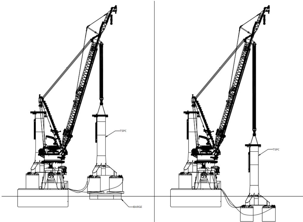
Step 4: Suction operation completed. Disconnect rigging, retrieve air hoses and suction pumps.
