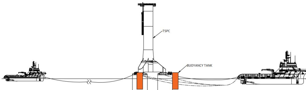
Step 3: Connect TSPC to JUP crane hook and lower TSPC till self-weight penetration reached. Disconnect hoses. Start suction operation.
