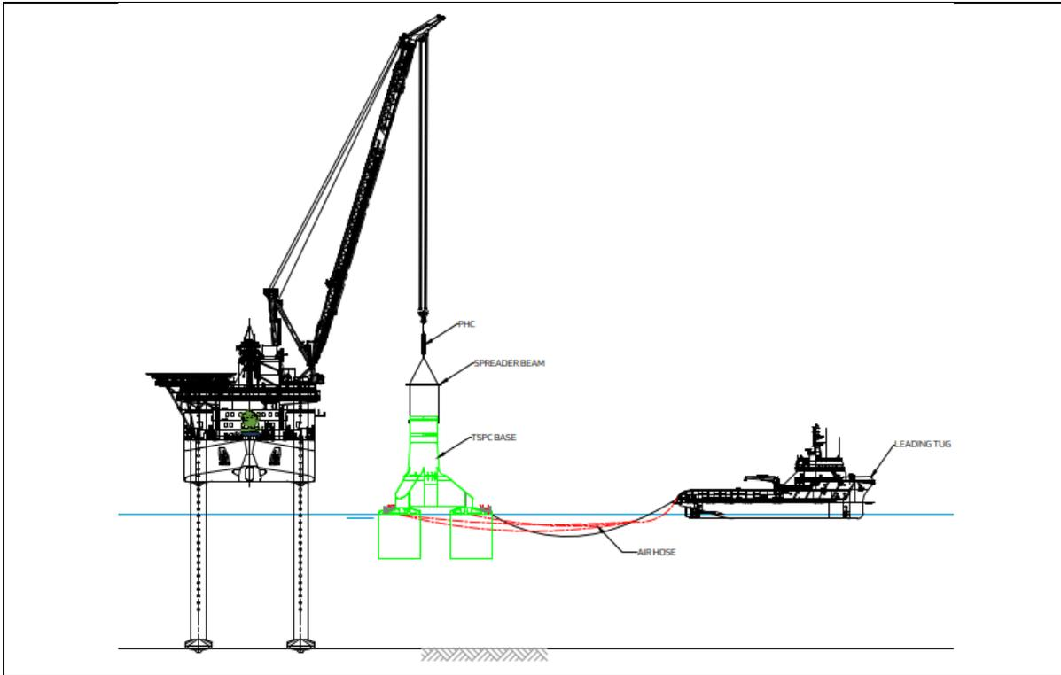
Step 4: Lower TSPC base till self-weight penetration reached. Disconnect hoses. Start suction operation.
