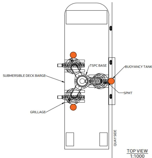
Step 2: Tow out the free-floating base with tugs directly to field OR tow out semi-sub barge to deeper waters, submerge the barge and tow out free-floating TSPC base.
