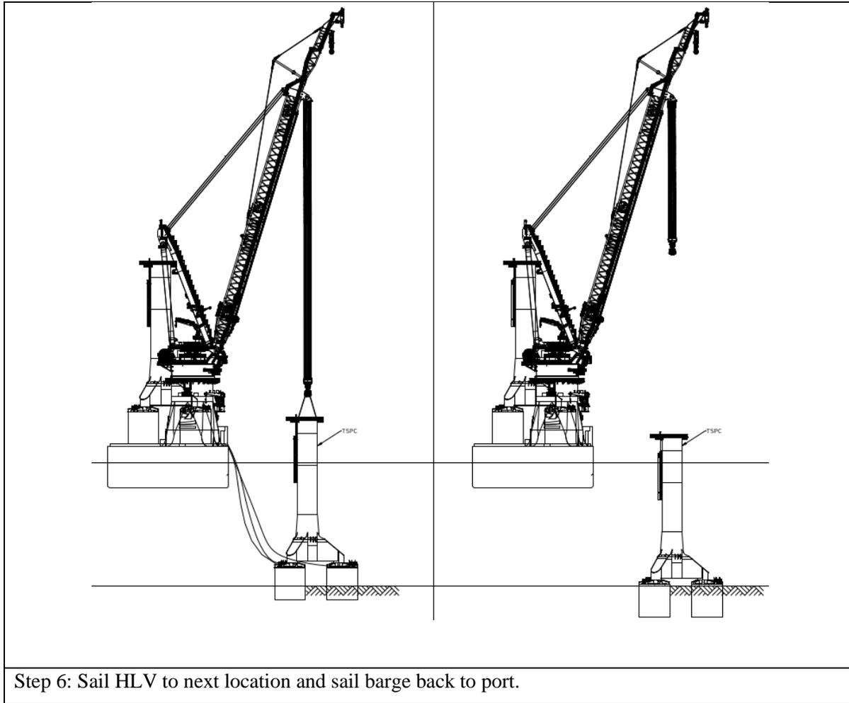
Regarding demobilization, TSPC can be retrieved relatively easily by applying a reverse effect on the suction buckets, allowing the structure to be fully removed, minimizing the environmental impact compared to other foundation types.
