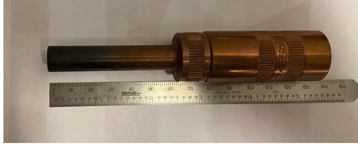
Figure 67. Narrow body torch used for deep groove welding.
