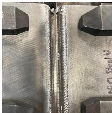
Figure 23: Underside of 1st mild steel root pass after grinding
