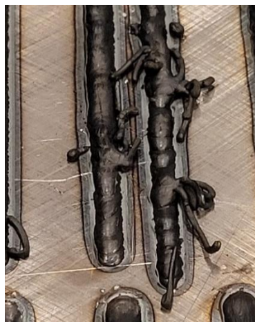
Figure 11: Cladding passes showing misalignment of wire feed – see wire portions that had fallen into to the weld pool
