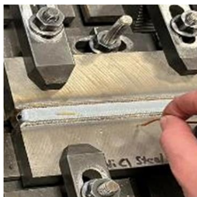
Figure 26: Weldment after all mild steel fill passes
