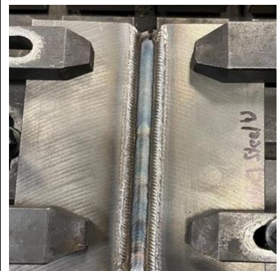
Figure 24: 2nd mild steel root pass on lower bevel
