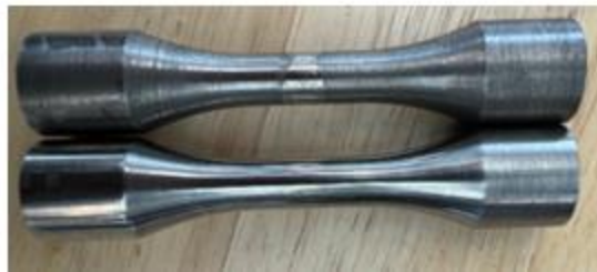
a) Cutting samples b). Turning into bars c). Profile making d). Polishing
