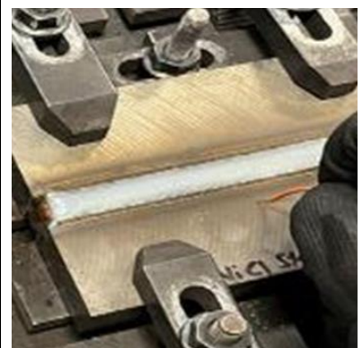
Figure 27: Weldment after mild steel cap passes
