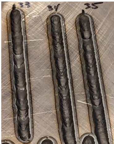
Figure 10: Cladding passes showing examples of balling and arcing – see the irregular surface of the weld
