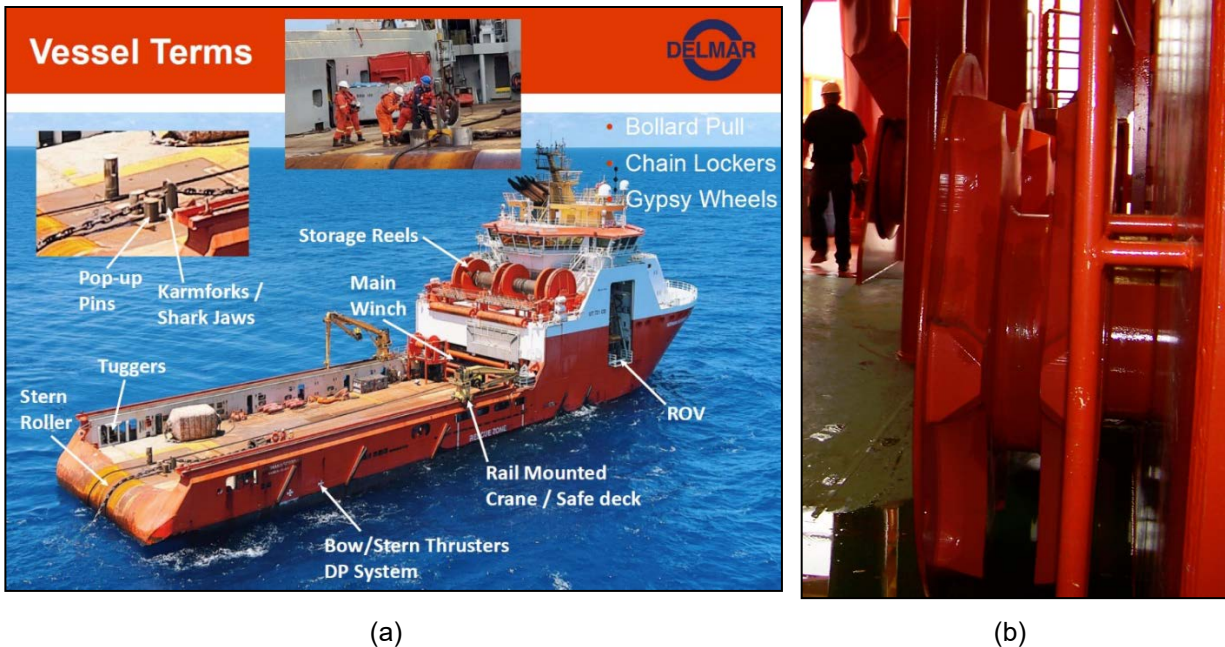
Figure 47. High-level overview of (a) an anchor handling vessel and (b) a whelp/gypsy wheel specific to one chain size.
