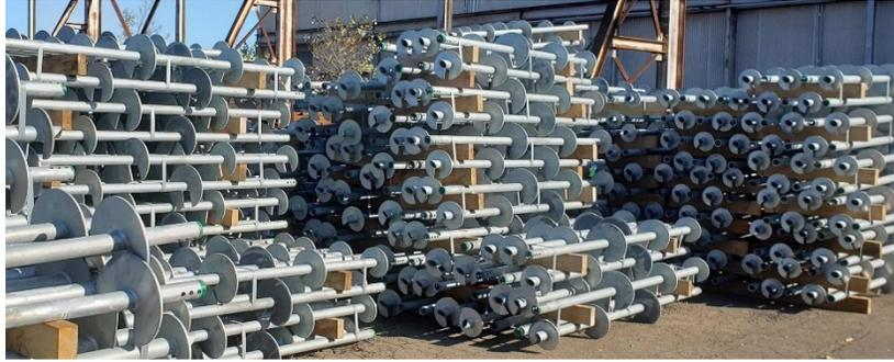
Figure 16. Mass produced helical piles
