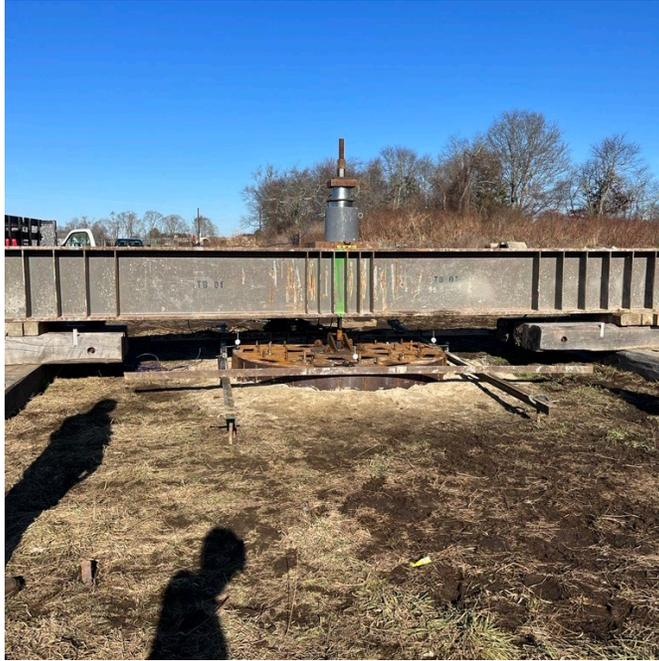
Figure 17: Vertical Test Configuration
