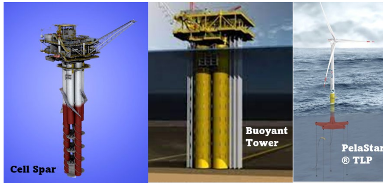
Figure 1 Cell Spar, Buoyant Tower and PelaStar® TLP 1
