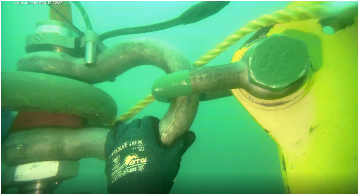
View of flounder plate on right, attached to a loadshackle, and the 4m IMS on the left.
