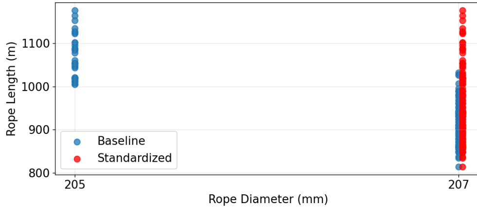
Figure 24. Rope diameter distribution between baseline and standardized designs
