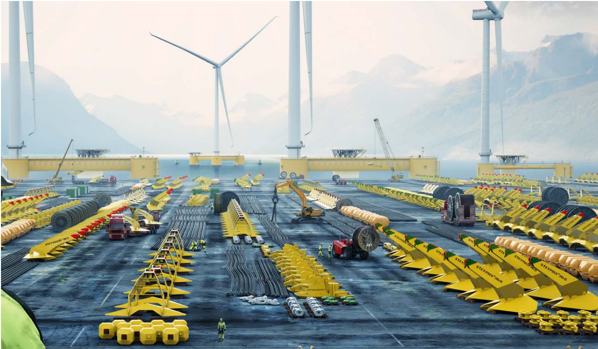
Figure 1. Illustration of stationkeeping components staged at port, including anchors, chain, spools of rope, and various accessories.
