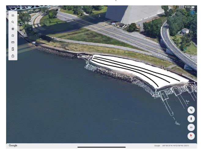
Figure 6-2. Overview of Owls Head to South Brooklyn Marine Terminal where the concept splits to allow cables to continue offshore (north) further into NY Harbor, or to continue onshore into Brooklyn (shown for three cables / circuits).
