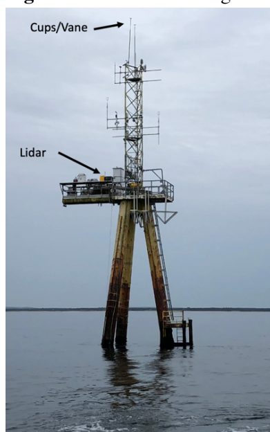
Figure 3. The ASIT in August 2021 with two lidars and the standard MORS-1 sensor suite deployed.
