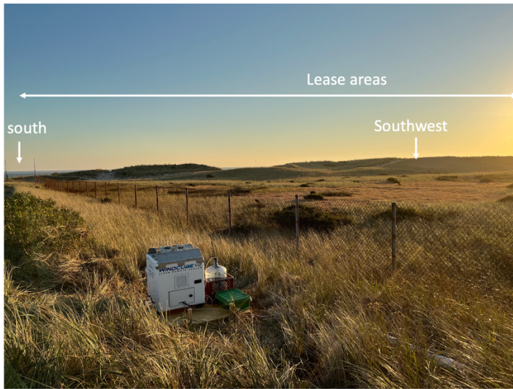
Figure 6. The WHOI Windcube v2.0 lidar stationed at the Nantucket test site, maintained between November 2021 and November 2022.
