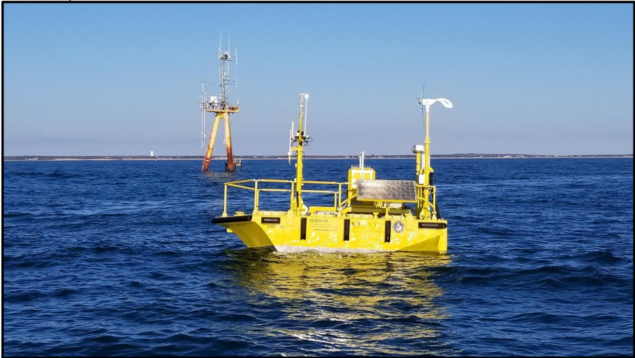
Figure 1: A lidar buoy owned by the U.S. Department of Energy on validation at Woods Hole Oceanographic Institution's Air-Sea Interaction Tower in January 2020.
