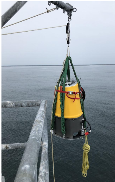
Figure 4. The ZX 300M Lidar being lifted to the ASIT in August 2021.
