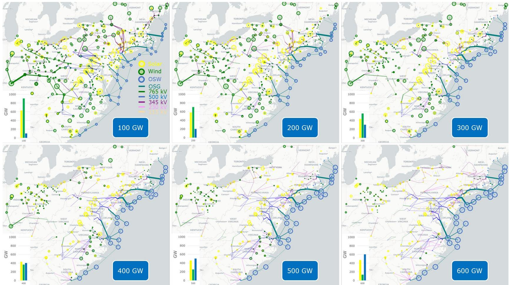
**Figure 3-4: Onshore & offshore added generation for OSW build-out levels of 100-600 GW in final year 2051.**
