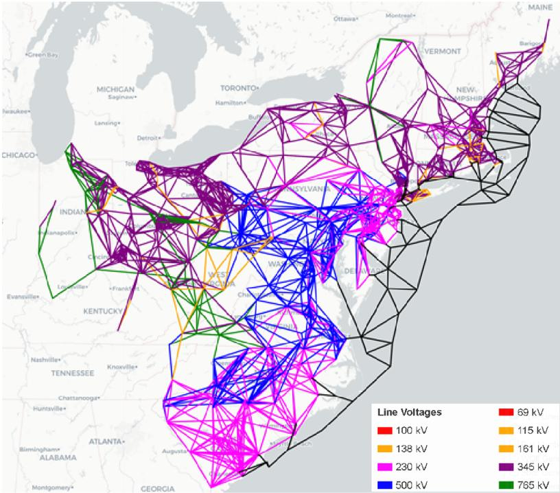
**Figure 2-2: Reduced 843-bus network with offshore grid template.**
