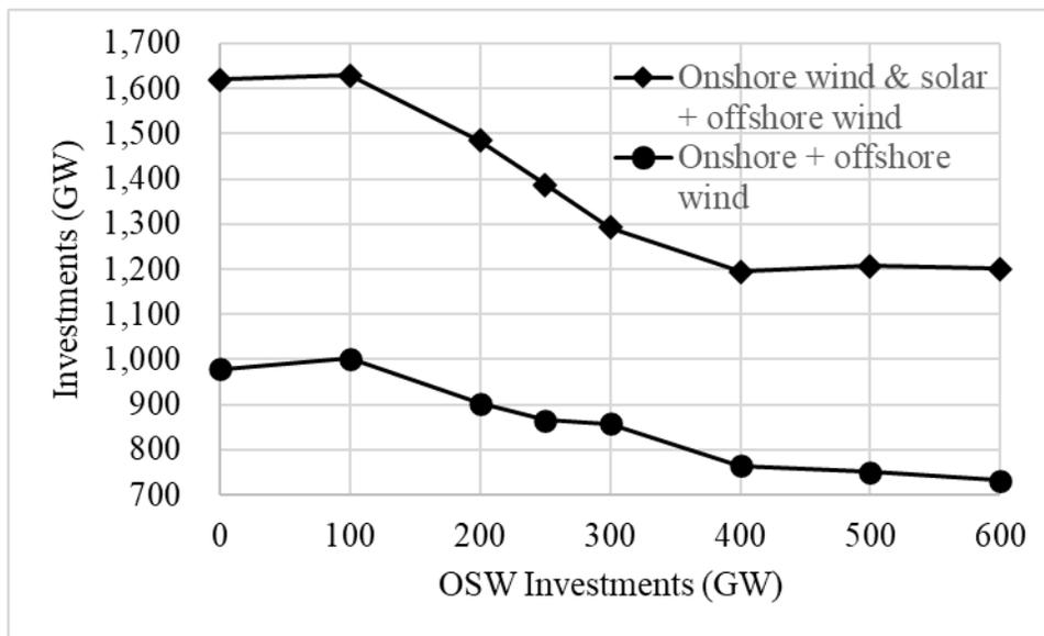
**Figure 3-6: Solar, onshore and offshore wind capacities in 2051 as OSW build-out levels increase.**
