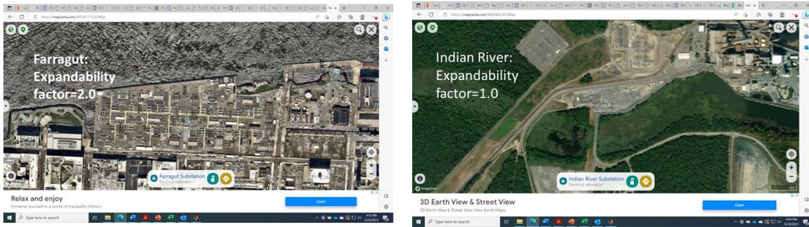
**Figure B-4: Illustration for two substations of satellite imagery used to estimate expandability factors (SEFs)**
