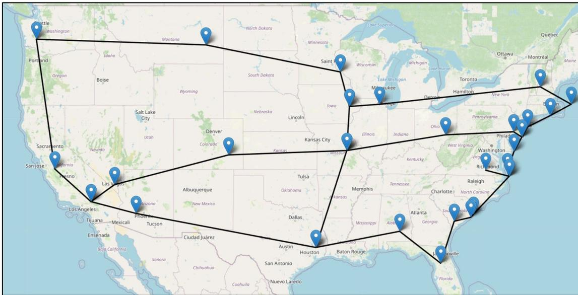
**Figure C-2. HVDC Macrogrid schematic**
