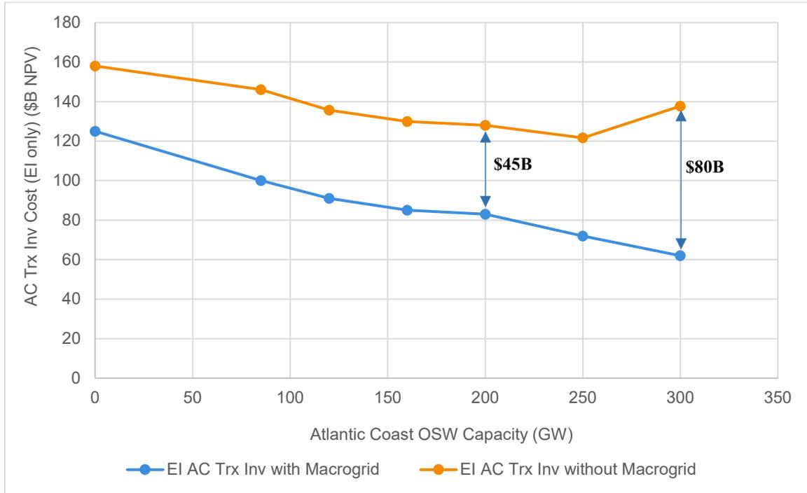
**Figure C-6. Plot of Atlantic Coast OSW capacity vs. AC upgrades required in EI, with and without the Macrogrid**
