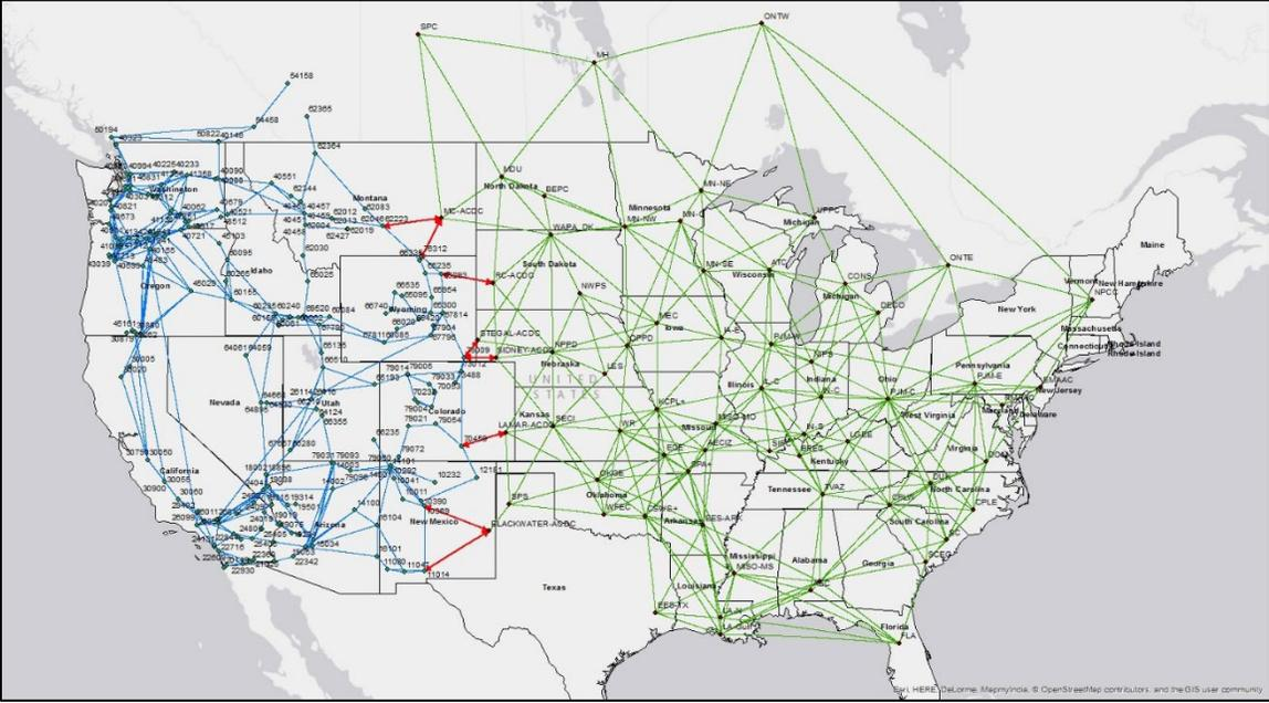
**Figure C-1. Illustration of 169 bus EI + WI reduced model**
