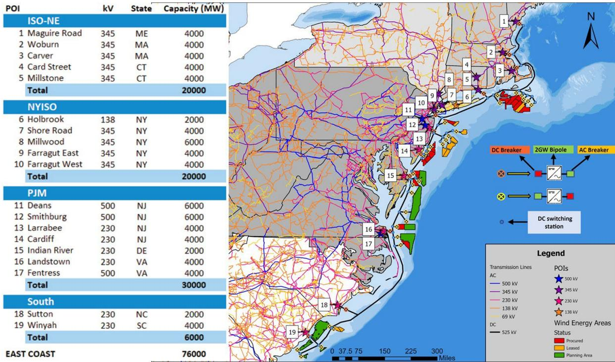
**Figure B-5: Results of POI assessment for 76 GW offshore wind level, by location**
