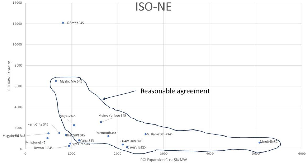
**Figure B-7: ISO-NE POI Comparison of Model 2 Capacities (MW) vs Model 1 Expansion Cost (\$k/MW)**
