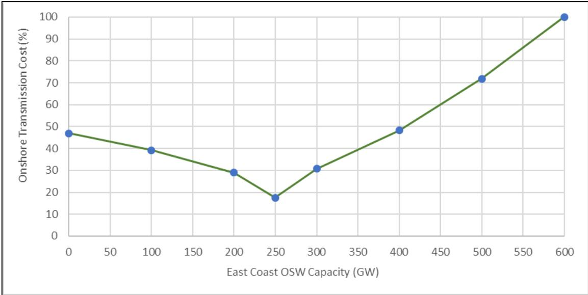
**Figure 3-2: Model 2, Onshore transmission investment cost vs offshore wind power capacity build-out (GW).**
