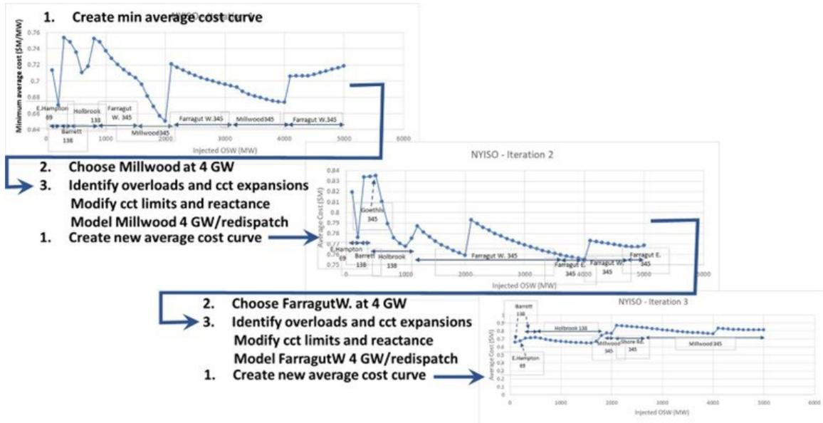
**Figure B-3: Illustration of two iterations of the heuristic optimization procedure**
