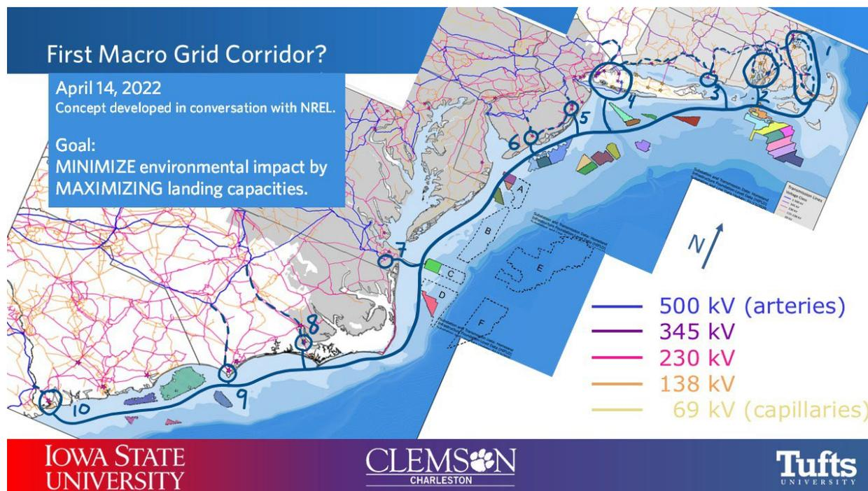
**Figure 1-1. April 14, 2022 sketch of an Atlantic Offshore Wind Transmission backbone.**
