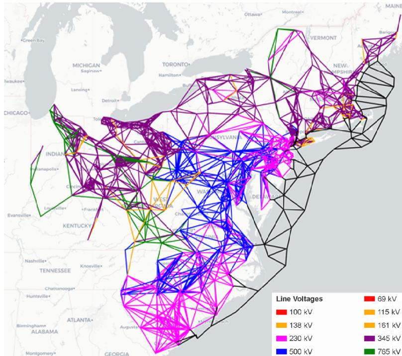
**Figure A-2: Reduced network with offshore grid design**
