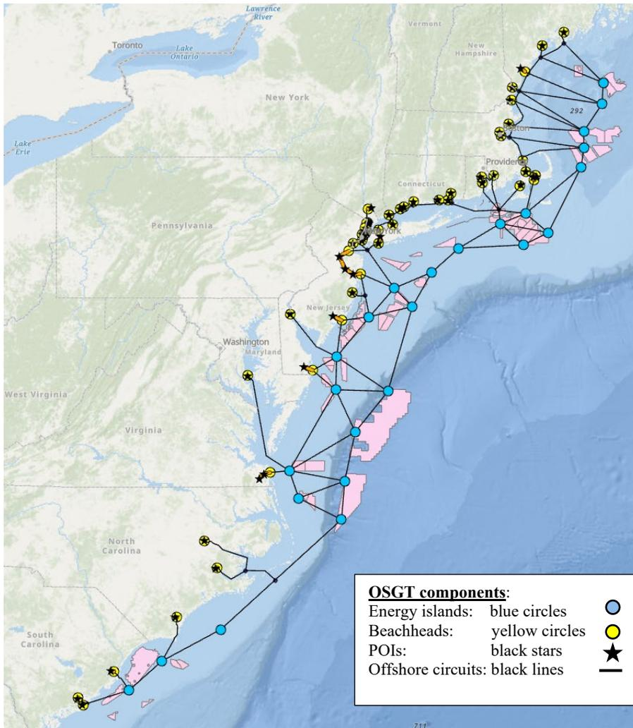
**Figure 2-3: Offshore grid template (OSGT).**
