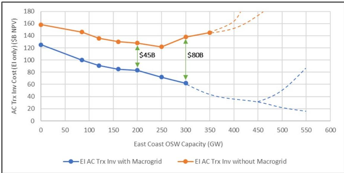
**Figure 3-3: Model 3, Plot of East Coast OSW power capacity build-out (GW) vs. AC upgrades required in the Eastern Interconnect (EI), with and without the Macrogrid.**
